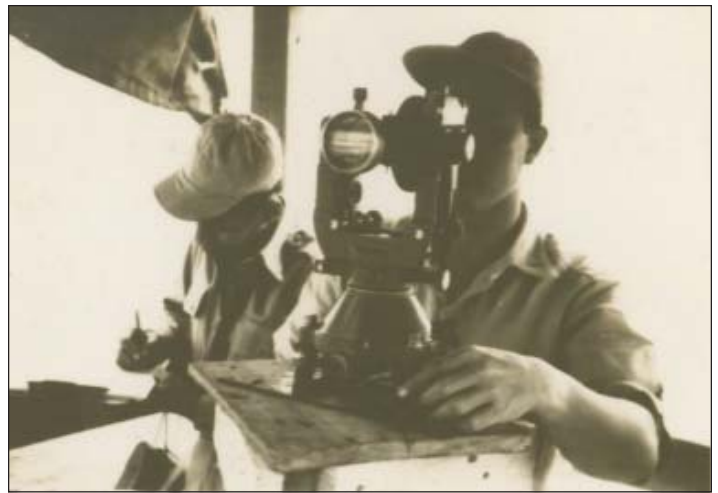
Observation in 1903 on station San Nicolas Beacon using Wild T-3 [Photo courtesy of the NAMRIA Library and Documentation Services]
