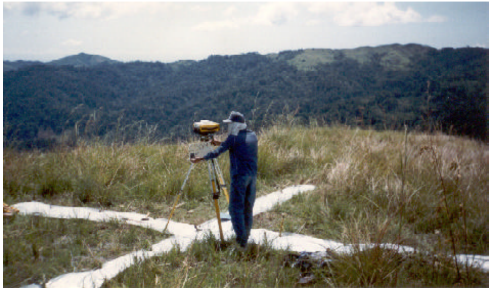
GPS observation over a signalized ground control point
