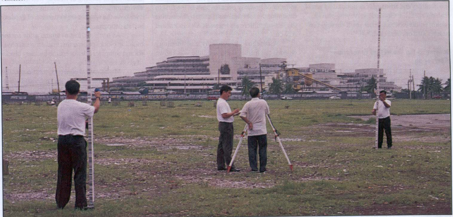
Surveyors calibrate their instrument prior to geodetic leveling work.
